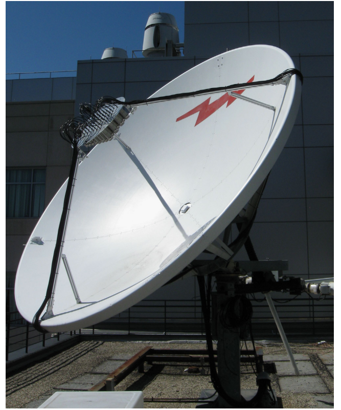
Fig. 1. The MIDAS telescope at the University of Chicago, with the 53-pixel camera at the prime focus of the 4.5 m diameter parabolic dish reflector.
